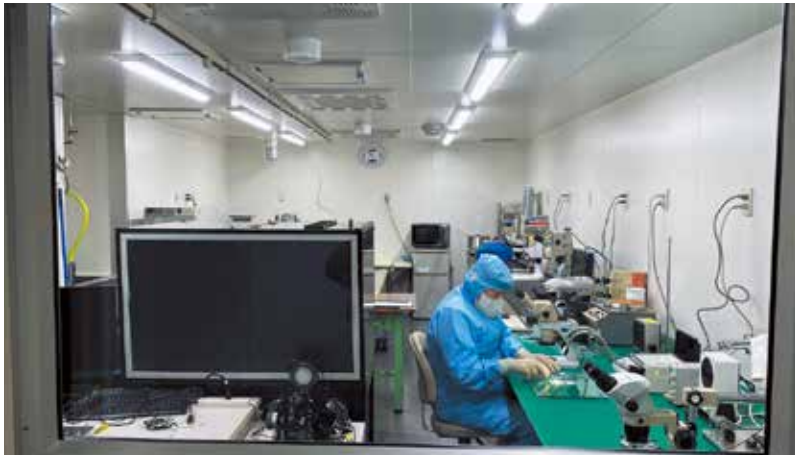
In a dust-free clean room, we perform adhesion, assembly, and prototyping evaluation of optical modules for small-diameter cameras and prism modules.
